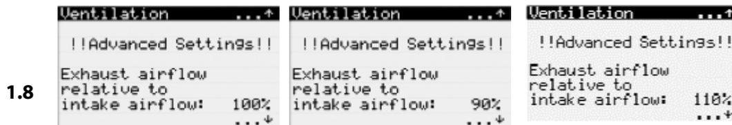
Figure 38 – Examples of options to adjust exhaust airflow.
