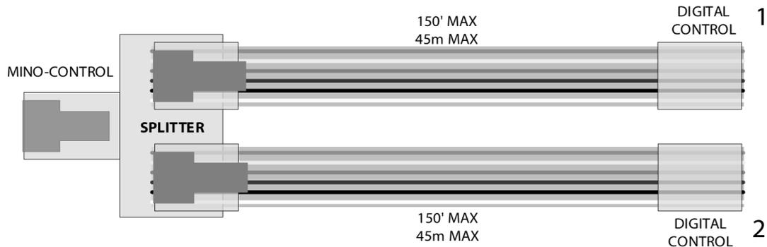
**Figure 22 - Cable configuration for two wallmount digital controls**
