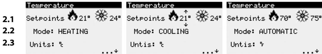
Figure 41 - Examples of options to adjust the temperature setpoint, mode and units.
