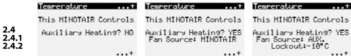
Figure 42 – Examples of options to adjust auxiliary (central) heating units.
