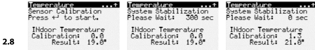
Figure 46 – Examples of options to calibrate the inside temperature sensor.
