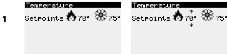
**Figure 31 - Examples of shortcut to adjust the temperature setpoint.**
