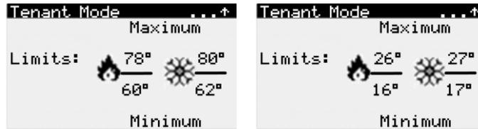
Figure 62 – Adjust the heating and cooling limits allowed in Tenant mode.
