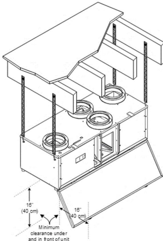
Figure 14 – Mounting the MINOTAIR using the floor joists.
