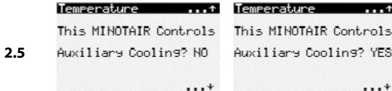
Figure 43 – Examples of options to adjust auxiliary cooling units.
