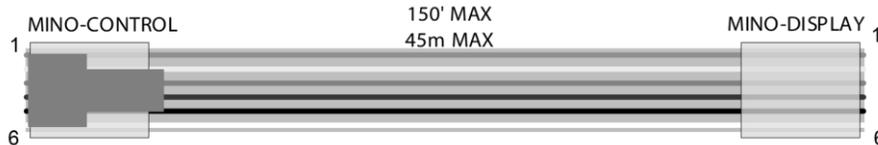
**Figure 20 – Cable configuration for a single wall mount digital control.**
