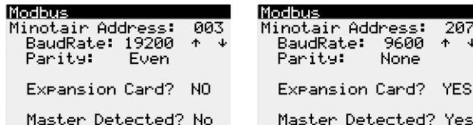
Figure 63 – Examples of options to adjust Modbus settings.
