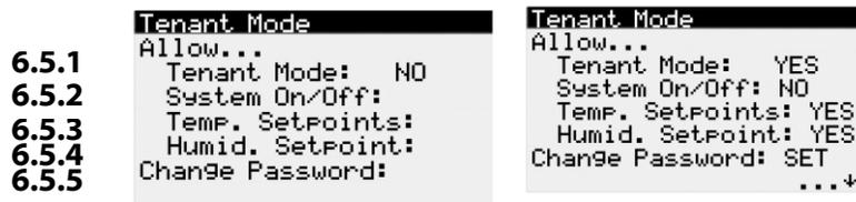
Figure 60 – Examples of options to adjust tenant mode settings.
