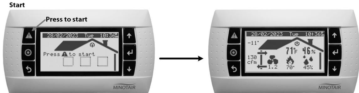
Figure 29 – To turn on the MINOTAIR, press  $\Delta$ .
