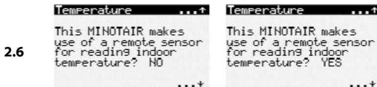
Figure 44 – Examples of options to adjust a remote sensor.
