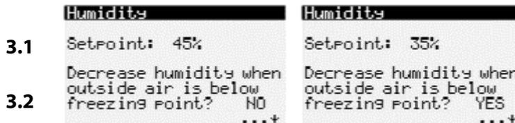
Figure 48 – Examples of options to adjust humidity settings and automatic winter adjustment.
