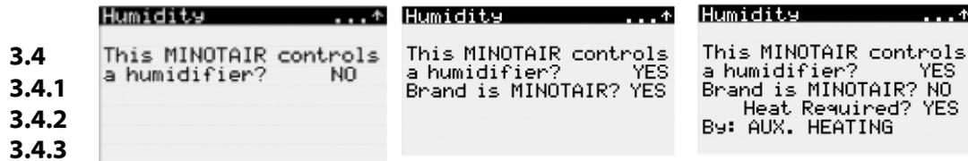
Figure 50 - Examples of options to adjust humidifier settings.
