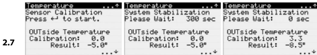
Figure 45 – Examples of options to adjust outside temperature calibration.
