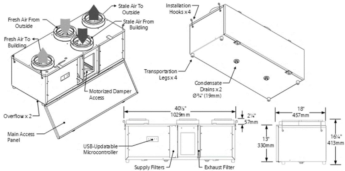
**Figure 3 – External overview of the device.**
